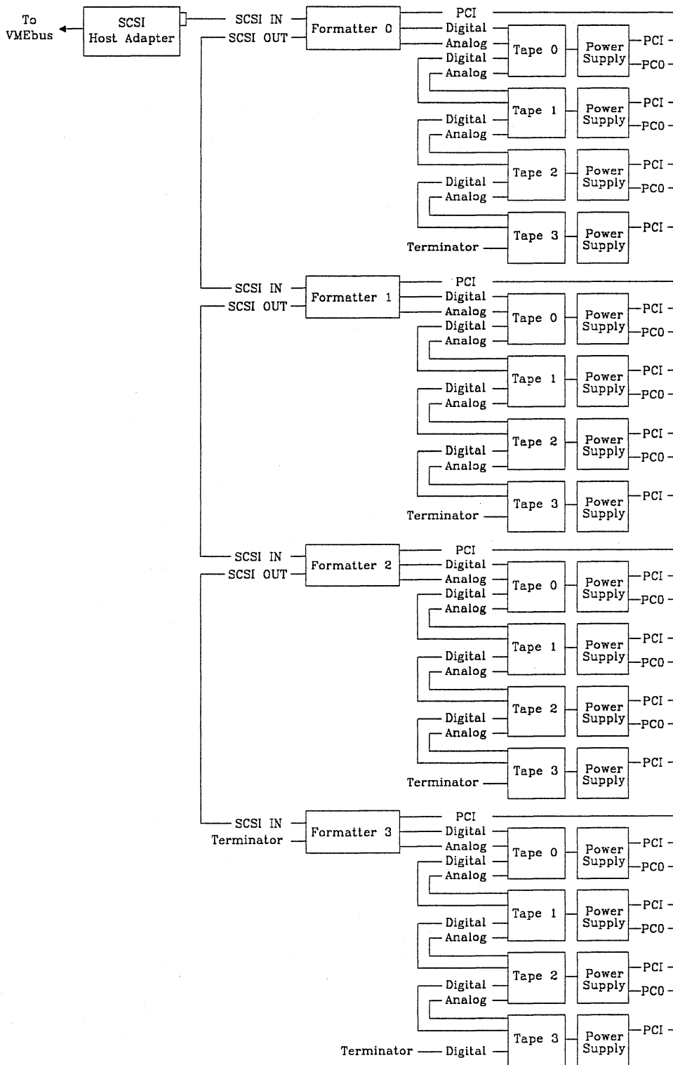
Figure 1-1, CONVEX 3480-Compatible Cartridge Tape System Block Diagram
